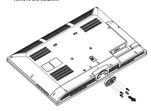
4 Attach the wall-mount bracket to your TV using the mounting holes on the back of your TV. See the instructions that came with the wall-mount bracket for information about how to correctly hang your TV.
